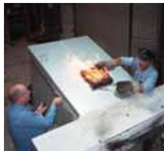
Example of fire test for roof
